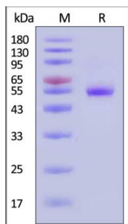
Rat LAG3, His Tag on SDS-PAGE under reducing (R) condition. The gel was stained with Coomassie Blue. The purity of the protein is greater than 90% (With [Star Ribbon Pre-stained Protein Marker](#)).
